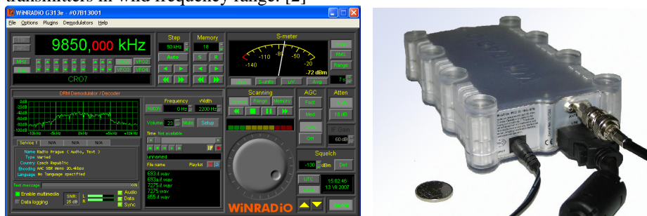
Fig. 4. Winradio WR G313 – the remote software and the hardware parts
